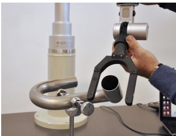
Pipe measurement by laser fork
