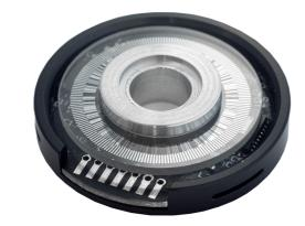
This is a high-resolution, singleturn absolute encoder with a 20 Bit BISS-C interface. The encoder consists of several optical reflectance sensors arranged at an angle of 180 degrees to each other. This allows to
