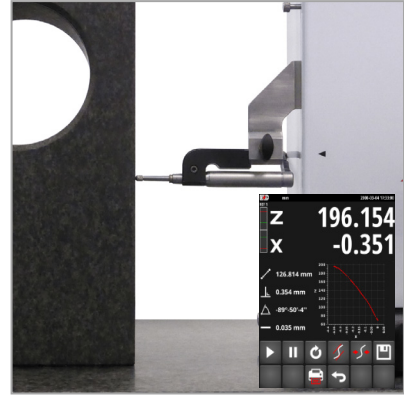
Perpendicularity measurements with electronic probe (TA-IH-126, TA-MS-101)
