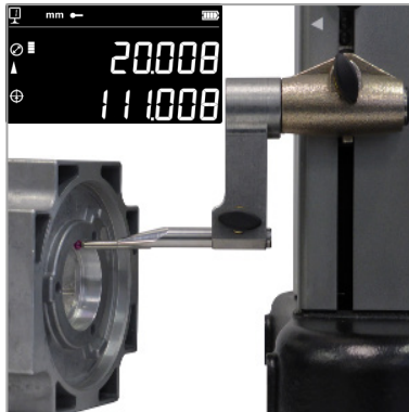
Simultaneous display of diameter and centreline (TA-IH-135, TA-MI-101)
