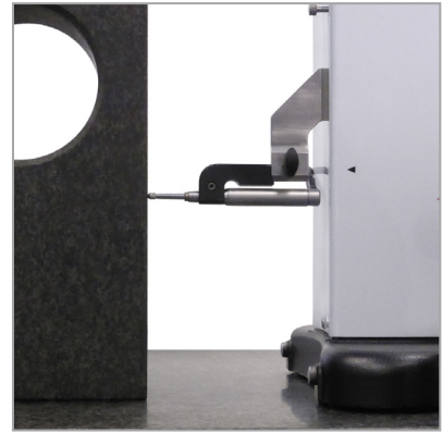
Perpendicularity measurements with electronic probe (TA-IH-126, TA-MS-101)
