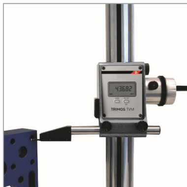
Diameter measurement with bidirectional probe (TVM4)
