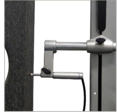
Measurement of perpendicularity with electronic probe (V6) (TA-IH-136, TA-MS-101)
