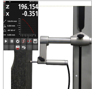
Measurement of perpendicularity with electronic probe (TA-IH-136, TA-MS-101)
