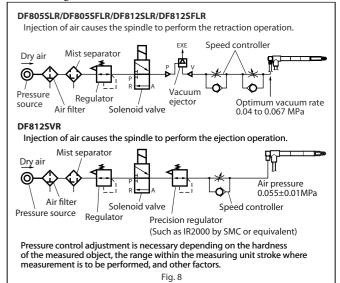
If the spindle ejection speed is too fast, an error may appear on the display the moment that the workpiece is touched. Excessive impact may dislodge the retainer inside the bearing, causing the measuring range to be reduced. In this case, use a speed controller as shown in Fig. 8 to adjust the spindle speed.
