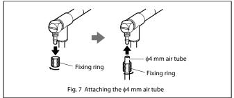
Place the end of the air tube in a location where it will not come into contact with water, oil or dust.
