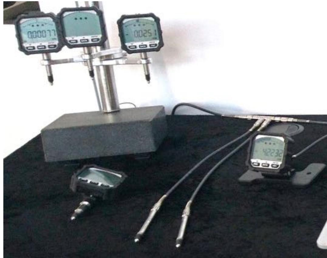
Measuring station with several SD1 dial gauges
