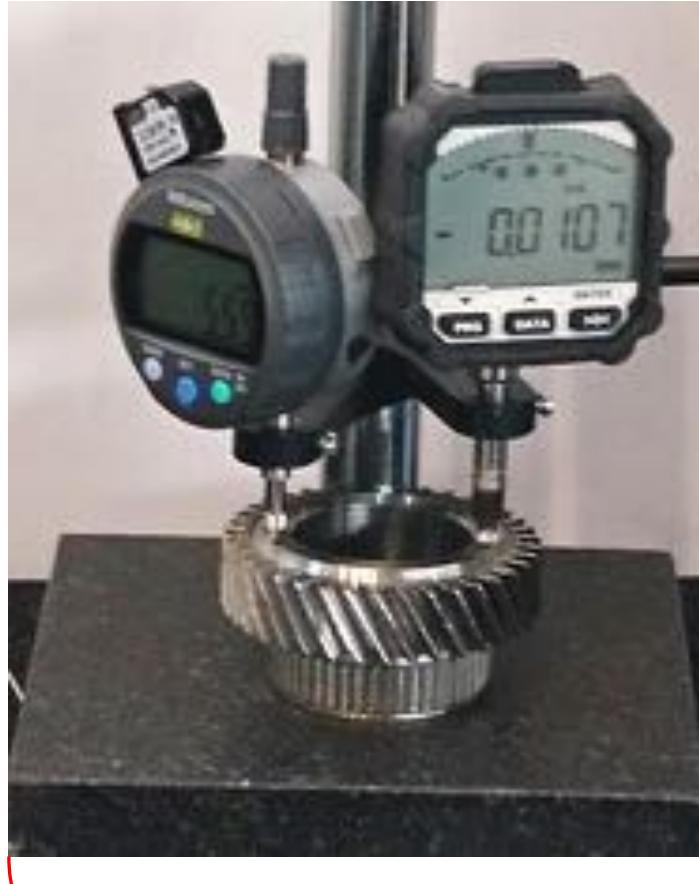
Radio measuring station with SD1 and Mitutoyo dial gauge
