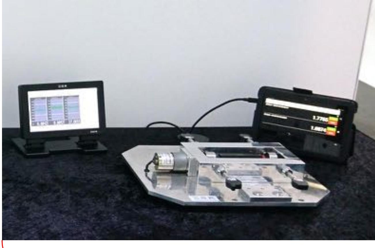
IMS-5S probes connected to a CD70 / tablet via radio
