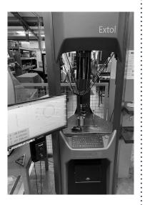
The successor to the company's award-winning Xtreme CMM, the Extol benefits from a smaller footprint, yet increased measurement volume. Ergonomics have been a significant design factor - ample access means the CMM is ideal for batch inspection and automatic loading.
