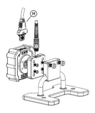
(H) 3i-USB [F420 010] Triple -I connection cable for USB interface
