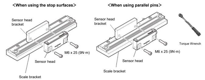
Insert the SZ26 between the sensor head and the scale. Then fix the sensor head under condition of light contact at both ends.
