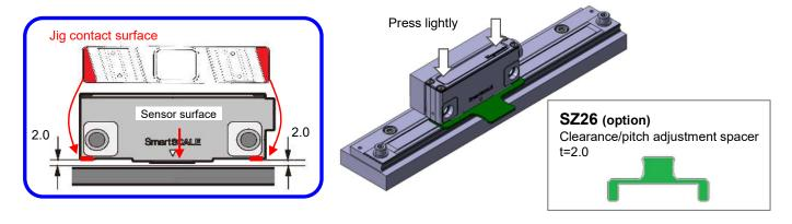
Remove the SZ26 and make sure t=0.1mm gauge should enter the gap and t=0.25mm gauge should not enter the gap.
