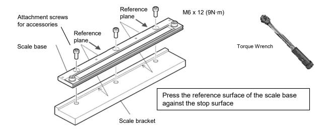
**Note**: In case of use of other non-supplied screws , the screw head may project from mounting surface. Do not use a screw with large "R" or no screw threads at base part as shown below.
