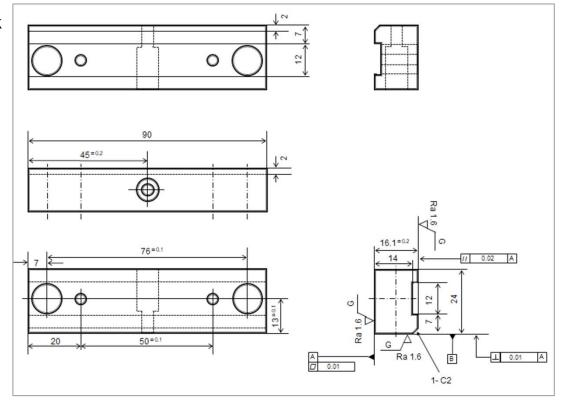
Note 1: No burrs on each surface, chamfering of unspecified corners is C0.5 or less Note 2: For assembly, 3 hexagon socket head bolts M4x16
